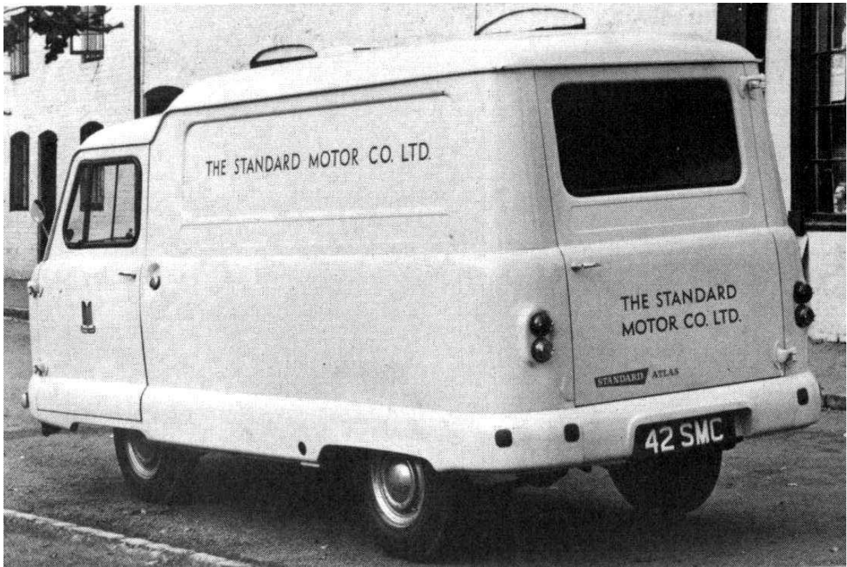
The utterly appalling Standard Atlas van of 1958 with its 948cc Herald engine, drum brakes and sliding doors that regularly fell off their runners under heavy braking!! The Atlas ‘morphed’ into the Leyland 15 and 20 and was available as van, truck or crewbus. it used a 1670cc or 2138cc Zenith carb Vanguard engine, had front disc brakes and hinged doors - and was a much better product all round than its predecessor.
