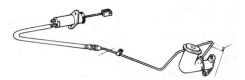
While under the car bleeding the system you might notice that the clutch arm doesn't move very far while the pedal moves a large distance from full out to full in. What is going on? To answer that we examine the pedal and hydraulic systems and apply some high school physics.
