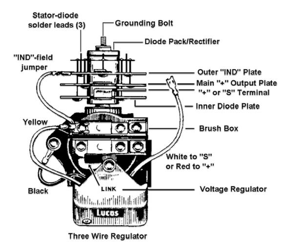
Remove the spade connectors that attach the regulator (and brush box) to the diode pack. Remove the two screws that retain the brush box/regulator assembly; you need to do this to check the brushes and get to the slip rings of the field windings.
