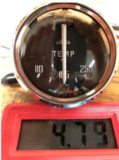
Fig 3: Mid-scale calibration verification
