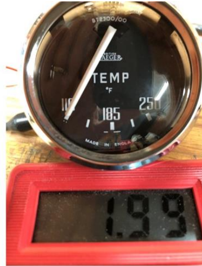
Fig 2: Low (2.0V) calibration adjustment
