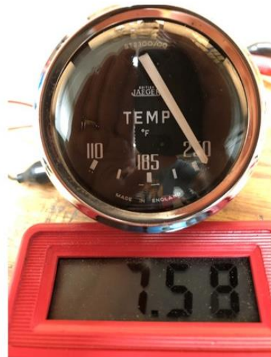
Fig 4: High (7.6V) calibration adjustment
