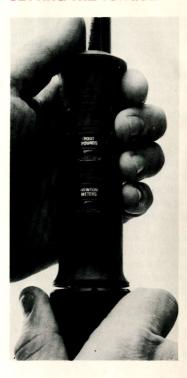
Before adjusting the wrench to the desired torque setting, **make sure** that you are using the correct torque units. Torque values may be given in units of Inch Pounds, Foot Pounds, Meter Kilogram or Newton Meters. Your **DIGITORK™** wrench is calibrated in Foot Pounds (upper window) and Newton Meters (lower window).
