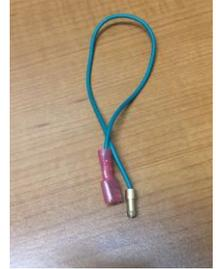
Next make the 2 jumper wires for the switch. The Alpine and Tiger both have a wiring harness junction under the dash on the driver's side which makes this solution very simple. Cut 2 wires 10" long and place a female spade type terminal on one end and a male bullet connector on the other.
