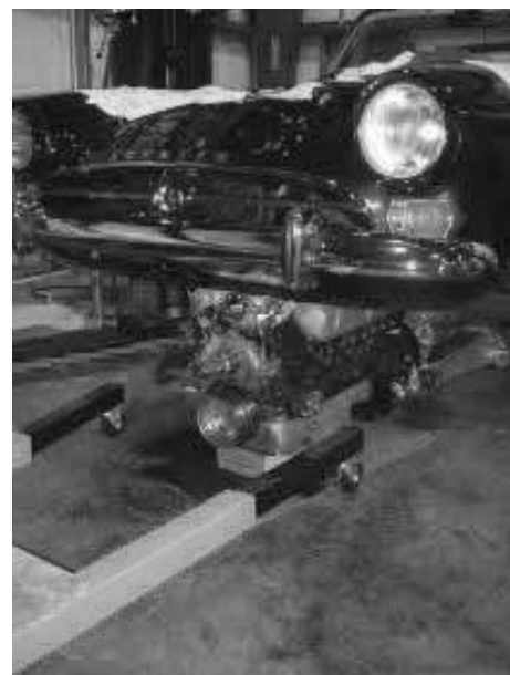
17 Remove the motor mounts and carefully lower the engine to the floor.
