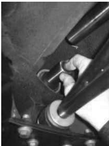
11 Remove the driveshaft. Be sure to plug the transmission output shaft. It will leak fluid. You can use an old yoke or welded plug like shown here.
