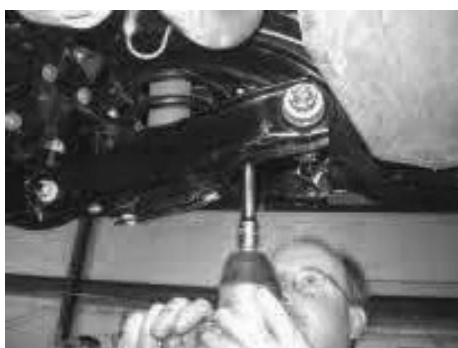
12 Remove the four 3/4" bolts holding the crossmember in the car.
