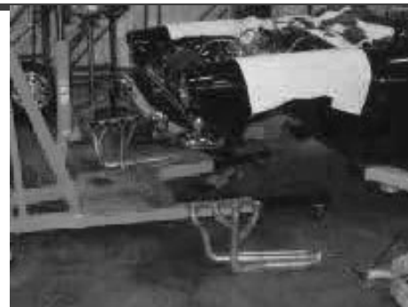
16 Header removal is generally a two person job to keep from chipping your paint
