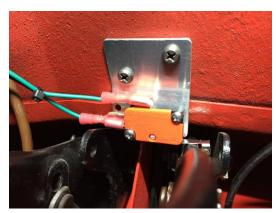
mechanical switch. After looking around for a suitable plunger type switch I decided to take a different approach and use a micro-switch. The nice thing about these switches is that they are easily sourced, low cost, reliable and best of all can be configured for "normally closed" operation. This switch solution requires no cutting or splicing of wires and only 2 holes need to be drilled.
