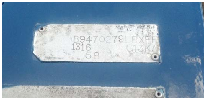
Figure 7: Style 4: Alpha and first five numeric characters of VIN, Build Series and Engine Series are in sans serif font. (Note: no gap in Build Series data; see Variant 2, below)
