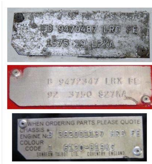
Figure 11: Style 7: Raised letter examples of VIN tags (top French, middle USA, bottom British; Rootes1.com 2016).
