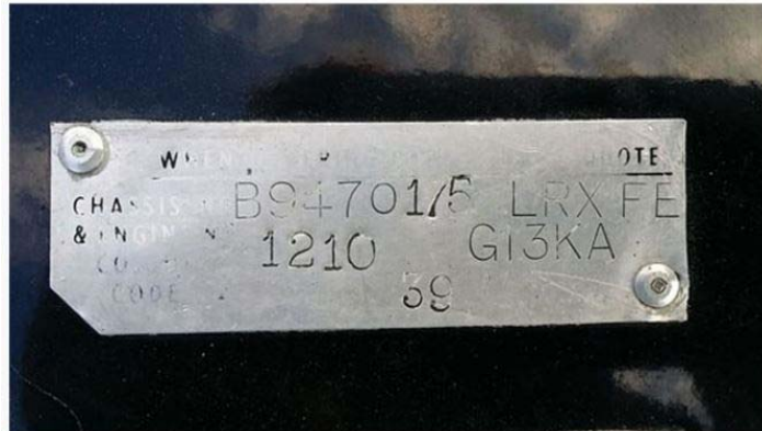
Figure 6: Style 3: Alpha and first four numeric characters of VIN, Build Series and Engine Series in sans serif font. (Gap in Build Series data; see Variant A, below)
