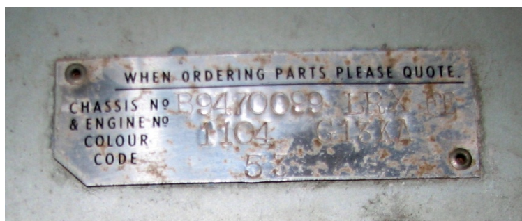
Figure 4: Style 1: All serif font (highest Style 1 VIN tag in the sample) (Note gap in Build Series data; see Variant A, discussed below)
