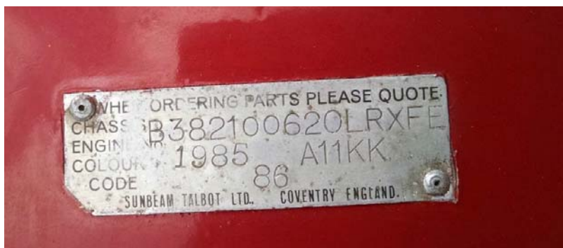
Figure 9: Style 5: Alpha and first six numeric characters of VIN, Build Series and Engine Series in sans serif font (last Style 5 VIN in the sample) (Note: no gap in Build Series data; see Variant B, below)
