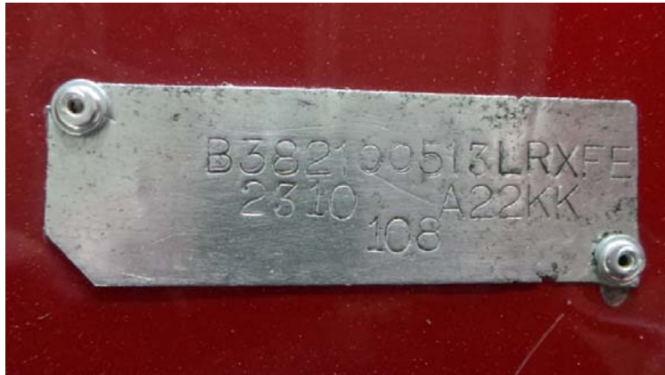
Figure 13: Style 5: Double misaligned stamp supporting a single punch scenario.
