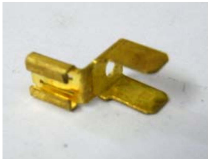
Figure 6. This spade doubler goes on your ignition switch on the terminal with the green wire. This will give you key switched power to operate your brake lights.
