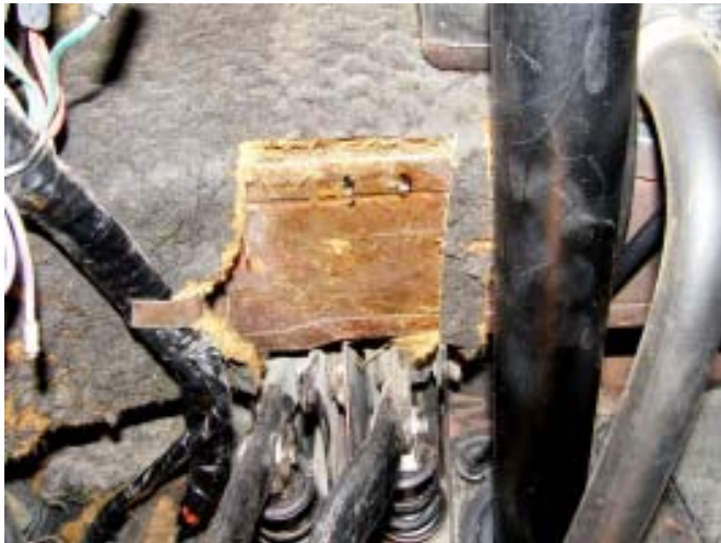
Figure 4. While holding the switch assembly in the position shown in Figure 3, mark the slots for drilling the holes to accept the mounting screws.
