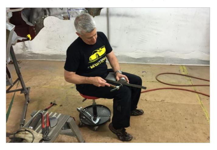
Once the flange is partly bent over, Tom rolls his round steel table over and hands me an Eastwood plastic hammer, which I use to complete the bend to 90 degrees. Doing this induces wrinkles and bends in the part and the flange, prompting more work on the shrinker/stretcher. Inevitably, the flange I was stretching needs some shrinkage to fine tune it and vice versa.
