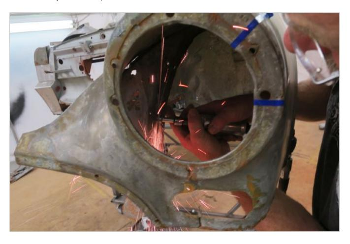
My task is to remove the front half of the driver-side engine-compartment sidewall. This part spans from the wheel opening on the bottom to the outer fender on the top and from the firewall at the back to near the radiator support in the front. It was kinked and damaged in the frontal shunt. Step one: Locate and drill out what turn out to be 11 spot welds attaching the front of the panel. Tom has a set of mono-taskers for that called Rotabroach cutters, sized to
