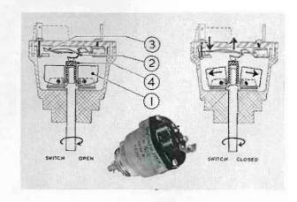
After removal of the switch, check that it is being driven and for possible end float at the spindle. This should be without '002" and may cause erratic operation if excessive.
