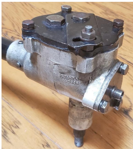
Burman , later (third) box design with adjuster & locking plate.
