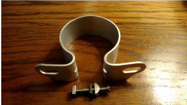
The BN2/100M coil brackets were very unique and looked like this photo above.
