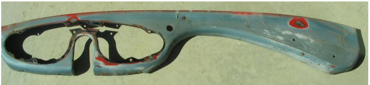
Early adjustable steering dash. Note the lack of the extra flange in the "U" shaped channel. M. Salter Photos.
