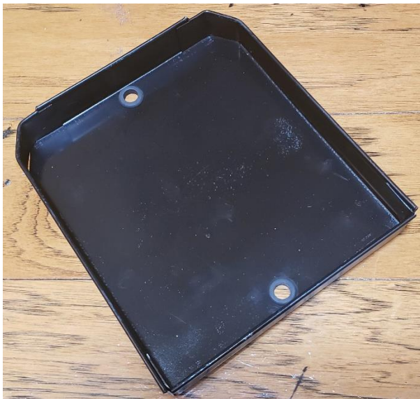
BN2 battery tray with integral angled corners, spot welded on one end. A more efficient design.
