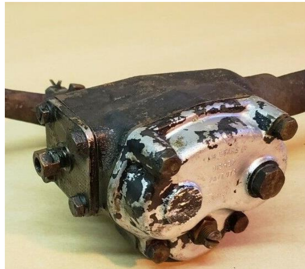
Cam Gears steering box with aluminum cover plate for later 100-six, 3000 cars. NOT used on BN2s!
