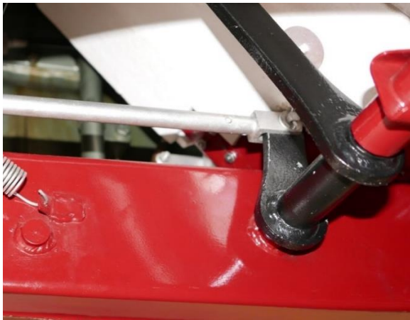
BN1/2-Brake pedal strengthened.
