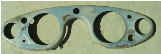
This is the instrument cluster section for the dash above. This would have had the "square" tabs on the back.
