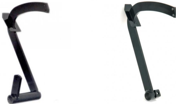
BN1 original brake and clutch pedals. Note how they are "butt" welded to the shaft.
