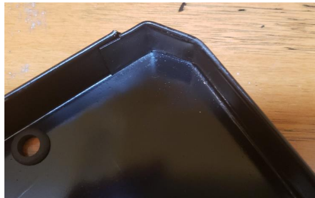
BN2 battery tray with integral angled corners, spot welded on one end. A more efficient design.
