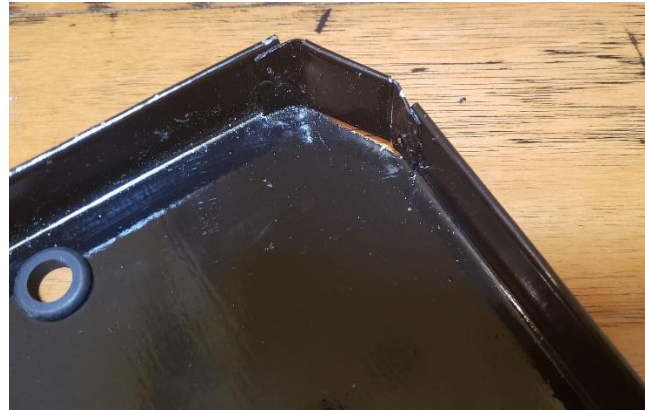
BN1 battery tray with separate pieces for the angled corners, spot welded in place.
