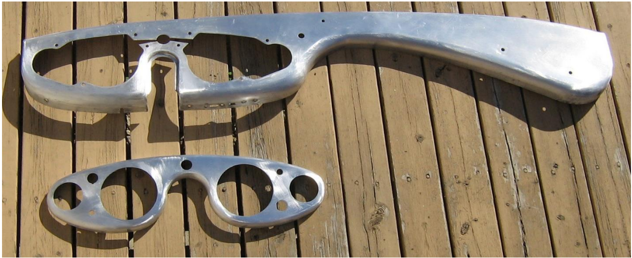
This type pictured above is the later type for cars with non-adjustable steering. Note the flange extension in the "U" shaped channel for the steering column. This type had the rounded tabs on the back, versus the square tabs.
