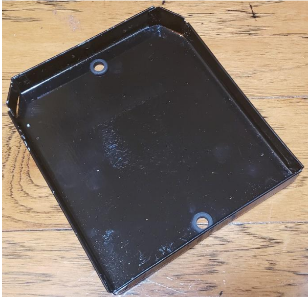
BN1 battery tray with separate pieces for the angled corners, spot welded in place.
