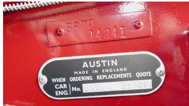
Oval metal (aluminum) chassis tag moved to firewall, underneath the batch/body tag.
