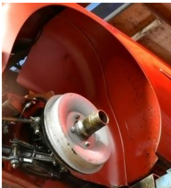
BN2 no. 13340 w/out front inner fender stiffening ridges.
