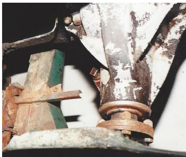
BN1 Hypoid Bevel rear axle filler pug on carrier. Note original red paint remnants on plug.
