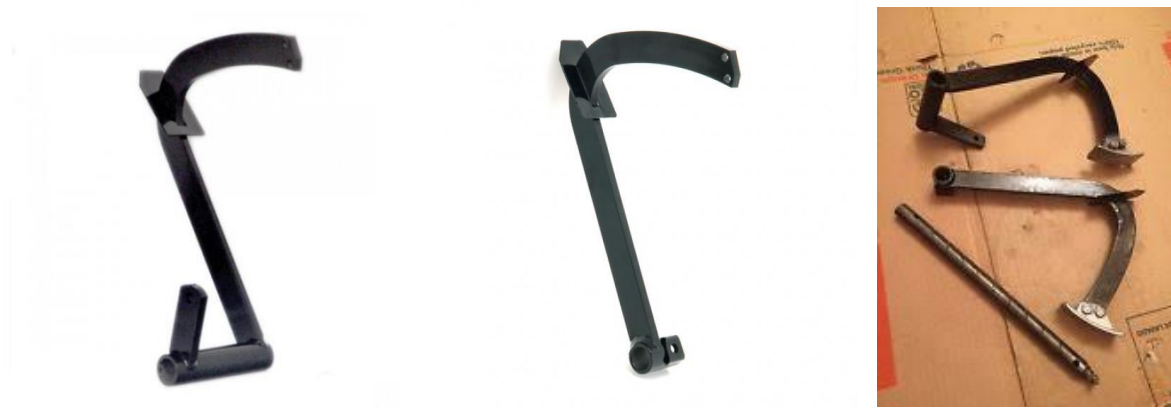
BN1 original brake and clutch pedals. Note how they are "butt" welded to the shaft.
