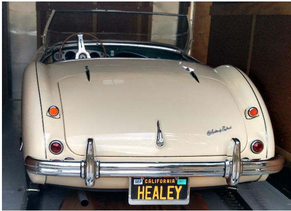
c222664, body no. 7197 built Jan. 11, '55. Reflector pods w/ Austin of England boot badge. Note original orange reflexes.
