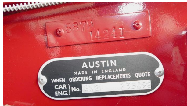
Oval metal (aluminum) chassis tag moved to firewall, underneath the batch/body tag.
