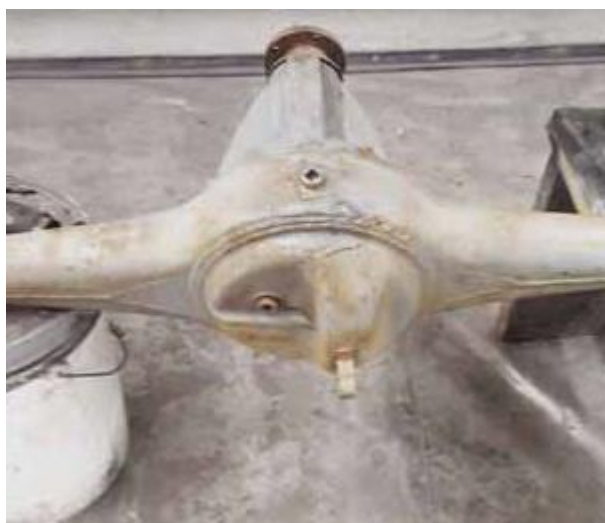
BN2 Hypoid Bevel rear axle filler pug on top of axle casing.
