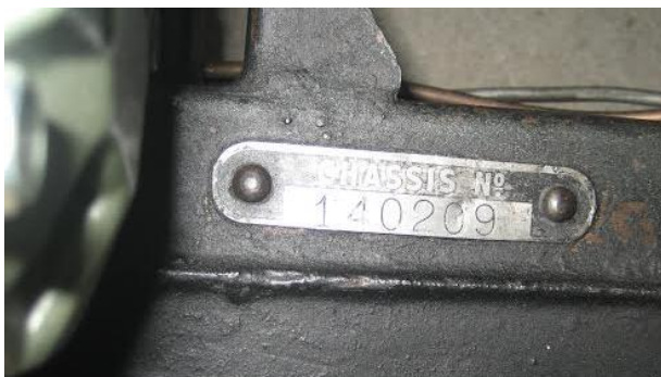
Chassis tag riveted to right frame rail.
