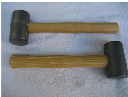
Accurate reproductions of the BN1/early BN2 lead knockoff hammer.
