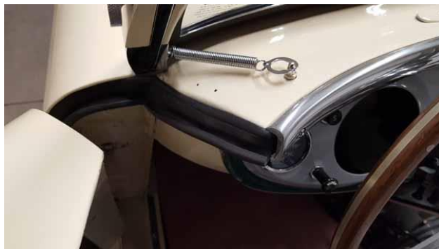
NOS improved scuttle seal installed. There was a BMC Service Bulletin on the modification.
