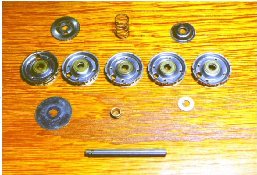
Figure 10. The disassembled parts of an "early" main odometer. The order of parts is from left to right and top to bottom. The brass keyed washers rest on top of each odometer wheel. These drag on the wheels and allow each to index when the wheel to the left releases the finger underneath.
