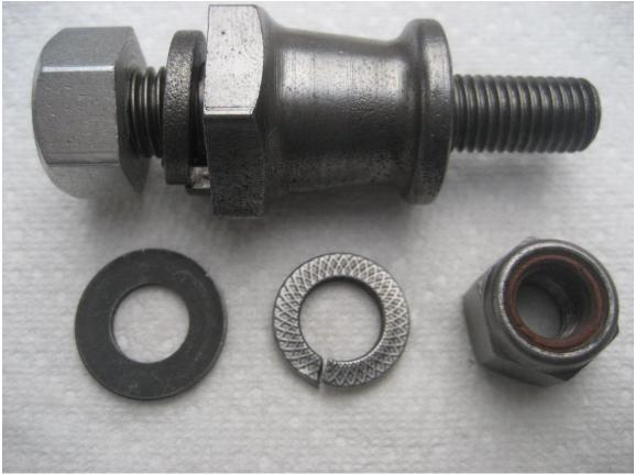
BN1/2 Generator pillar with a sampling of various fasteners; Bearing surface BSF nut, square profile spring washer, British pattern flat washer, "Basket weave" patterned spring washer and red fiber lock nut.
