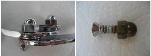
Cap or Acorn nuts. Used for the 5/16" seat back to frame hinge bolts. Also used on the 100s, 10-32 hood frame latch screws and 1/4" BSF latch pivot screws (pictured above).
