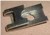
Spire nuts. Commonly used with special flat threaded hex nuts to attach fenders on British cars.
