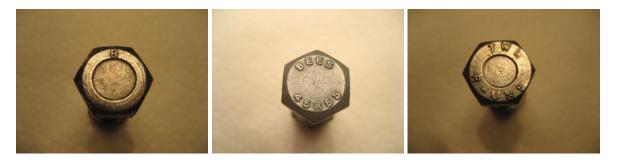
The R rating was used throughout the 1950s and early '60s when it was replaced by the "S" rating code. Most AH 100s, 100-sixs and early 3000s will have these "R" rated bolts.
