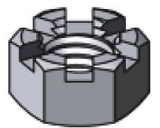
Slotted nuts are used in conjunction with a cotter pin on drilled shank fasteners to prevent loosening.
