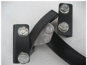
Two original 1/4" zinc plated bolts in the center and four 5/16" bracket bolts re-plated with Caswell's "Copy Cad".
