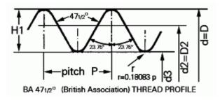
Similar to Unified numbered machine screws, BA threads are numbered, sequentially from 0 to 25, and the threads per inch are taken from a metric thread standard so they are very non standard when converted to inches. Also the numbering system is reversed from that the Unified numbered machine screws.
