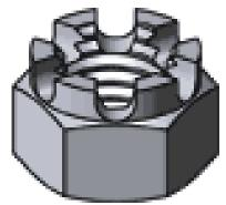
Castle nuts are similar to slotted nuts but with slots in a rounded section above the main nut.
