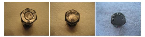
Starting after 1950, British High Tensile Steel bolts are numbered from "R" sequentially through "X", however we will concentrate only on the four grades found predominately on Austin Healeys, i.e., **R**, **S**, **T** and **V**, and not cover U, W and X.
