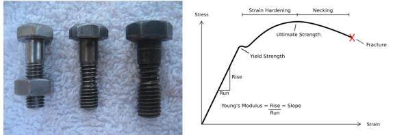
Bolts that have exceeded both their Yield Strength and Ultimate Strength, and have begun "Necking" (see the graph right). These examples are 1/4 & 5/16 BSF Grade "B" (Mild steel). The example on the far left has indeed stretched permanently since this is as far as the nut will smoothly screw onto the threads.
