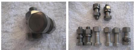
Engine to transmission 3/8" BSF hex bolts (6) and 3/8" BSF Dowel bolts (2).
