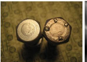
RSB-Regis Screw and Bolt w/ "R" strength rating. UNC bolt on left has no marking so it's a Grade 2
