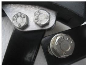
Original 1/4" zinc plated bolts on the left versus a 5/16" bolt on right re-plated with Caswell's "Copy Cad".
