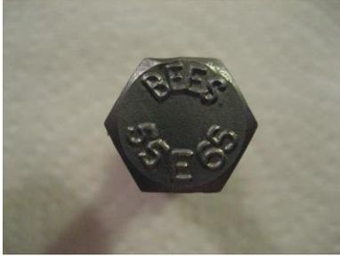
**C - Unknown**, but should be equivalent to Grade Q which I suspect may have a range UTS of 35/45 or more likely 40/50 TT.
