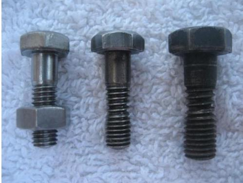
Bolts that have exceeded both their Yield Strength and Ultimate Strength, and have begun "Necking" (see the graph below). These examples are 1/4 & 5/16 BSF Grade "B" (Mild steel). The example on the far left has indeed stretched permanently since this is as far as the nut will smoothly screw onto the threads.
