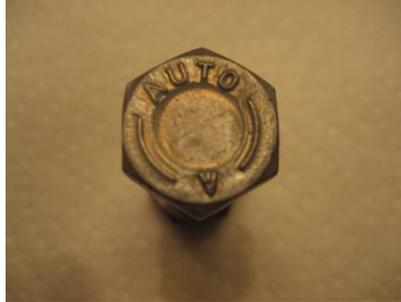
**W** - 70/80 TONS TENSILE, I have found several - 5/16 inch bolts with the "AUTO" vendor name with this rating (Austin Healey Sprite gearbox). The "W" rating corresponds to a 70/80 TONS TENSILE strength, as referenced in two obscure charts that I have found.
