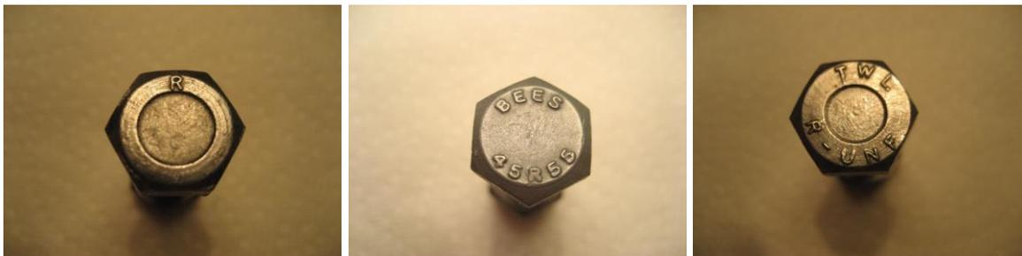
The R rating was used throughout the 1950s and early ‘60s when it was replaced by the “S” rating code. Most AH 100s, 100-sixes and early 3000s will have these “R” rated bolts.
