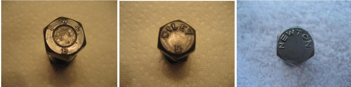
Starting after 1950, British High Tensile Steel bolts are numbered from “R” sequentially through “X”, however we will concentrate only on the four grades found predominately on Austin Healeys, i.e., **R, S, T and V**, and not cover U, W and X.
