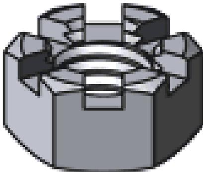
*Slotted nuts are used in conjunction with a cotter pin on drilled shank fasteners to prevent loosening.*
