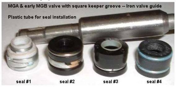
Notice with the installed views below the increased gap in the bottom retention band as the seals are stretched over the valve guide. Also note that use of these seals requires removal of the original oil deflector, in which case you should also get the later model spring cap with larger pilot diameter to fit the ID of the inner valve spring.
