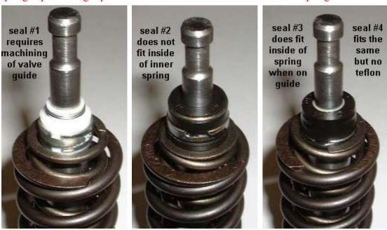
Early on I used some all-Teflon parts that would have almost infinite life under high temperature conditions. With not much experience I told the shop I wanted to use Teflon seals, and this is what they installed. See seal #1
