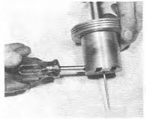
6.5A Extract the locking screw ...
