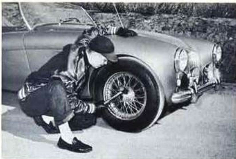
The wire wheels of Torne's special job are chromed but the production models come with painted wire wheels. Mel's car also has an all-aluminum body but the regular Austin-Healey "100", with an eye to traffic hazards, has steel fenders.
