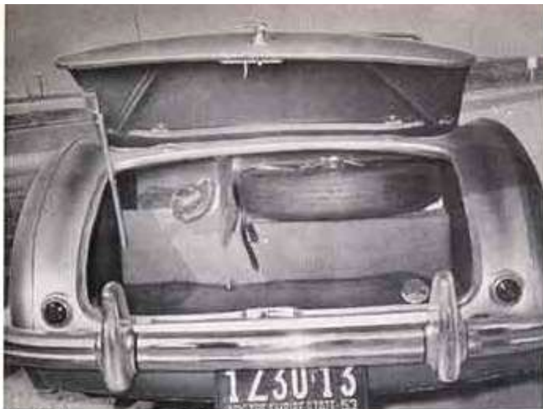
Despite the compactness of the Healey, the rear compartment affords plenty of room for luggage and spare tire. A master switch in the trunk cuts off all power.
