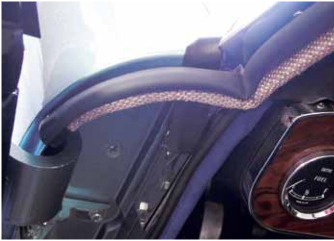
Photo 6: On BJ7s and BJ8s, the extra flap from the windshield-to-cowl seal will be tucked behind the windshield side pillar seal strip where it is attached to the rear of the front wing when the windshield and pillar seal are finally installed on the car.
