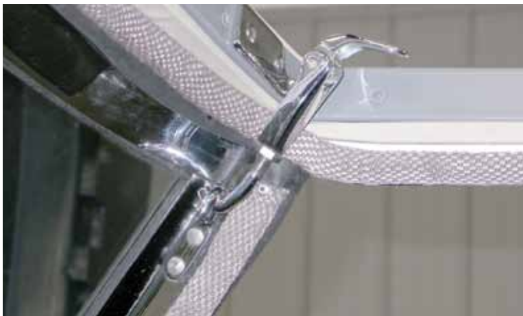
Photo 4: On BJ7s and BJ8s, the hook which the top latch engages is attached to the upper end of each windshield side frame using solid rivets. Solid rivets are also used to attach mounting brackets to the lower end of these frame pieces.
