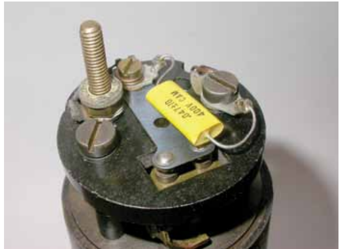
Photo 1: View of a 400v, 0.047uf capacitor "floating" above the points on an early type fuel pump. Note the washer/gasket on the terminal post to the left. Its purpose is to seal out air where the terminal passes through the bakelite cap. Capacitor connections are to the point's blade mounting screw (top) and pedestal mounting screw (right), which also serves as ground. The wires are sufficient to hold the capacitor in position.
