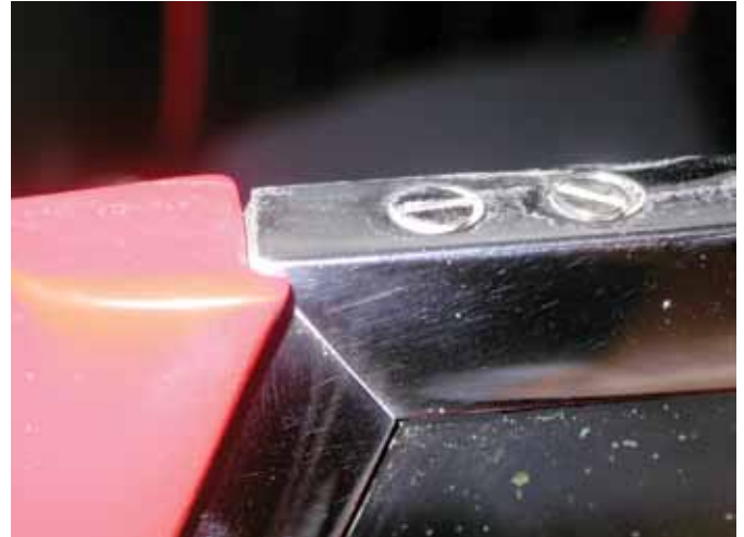
Photo 2: A windshield frame top mitered corner on a 100. This is typical of the configuration found on all roadsters. The top corner screws are the only ones visible on the finished assembly.
