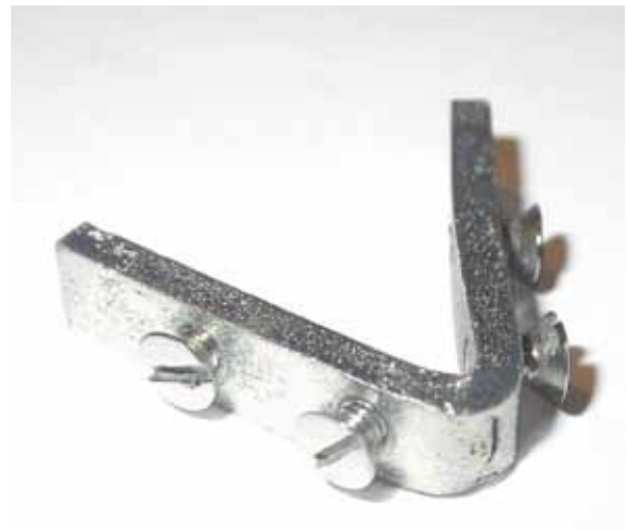
Photo 5: On roadsters (BN1 - 3000 Mk II) the lower corner brackets have sharper bends than the upper brackets. 4BA screws are used to attach these to the frame channels. These brackets were custom fit when the windshields were assembled at the factory, and should be restored and re-used, marking how they were originally positioned at each corner.
