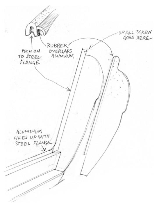
the steel flange on the car and the aluminum shut plate piece. It is pushed onto the upright steel flange only, but the Bristleflex is made so that the rubber flap on the outside overlaps the aluminum. This means you have to have some space between the aluminum and the steel. A lot of people have pushed these together and pushed the weatherstrip over the two.
