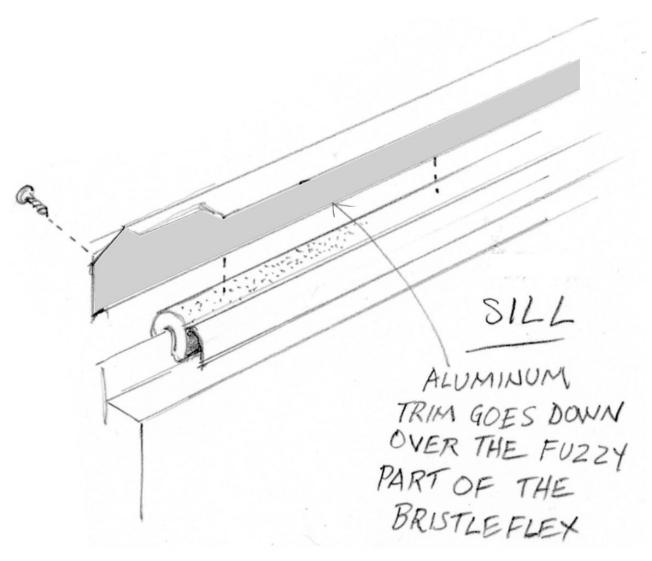
The other important thing is the way the aluminum sill trim goes on. It is screwed to the inner sill from the inside, but the top of the aluminum sill trim has to go down over the fuzzy part of the bristle flex. This holds it down and prevents you from kicking it off as you get in and out of the car.
