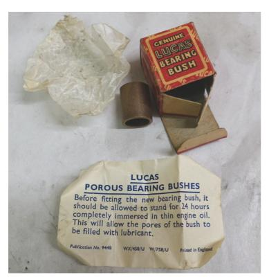
Original Lucas bushings were un-lubricated and come with instructions stating to immerse the bushing in oil for 24 hours before installation.
