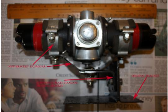
What I have done, as I hope you can see from the photo, is add an "L" shaped section of metal which is bolted to the original bracket. To this new section is bolted the ex-Jag bracket
