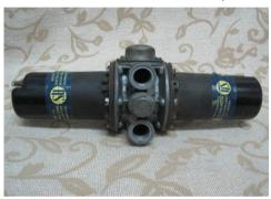
So far as I can see from visual comparison of the external view and the internal workings, this pump is two AUF 301 pumps siamized(?) in the middle. Anyhow, one buys two rebuild kits; one uses all of one kit and half of the other, the electric bits being duplicated and some of the mechanical/pumping bits being shared.
