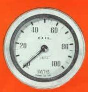
Oil pressure is vital and perhaps the most important in-strainent one can have on the dishboard is the gauge which indicates this pressure. Smiths oil pressure gauges work on the Bourdon tube principle and are robust and re-liable and are calibrated 0-100 lbs; per sq. Inch. An oil olpe line and tee piece are supplied with the gauge to acilitate connection to the engine.
