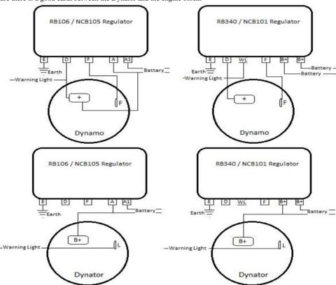
The NCB133 model 340 now replaces the old model RB310 type regulators. There are some physical differences in the two units but they are interchangeable. Model 310 was supplied with three terminal connections; B, F and D. It's replacement model RB340 has five; E, D, WL, F and B.
