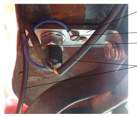
Brackets cut and drilled to fit from 1/4" x 1-1/4"- section heavy duty shelf brackets from hardware store.
