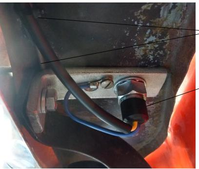
Crossover tube zip-ties to Inserted piece of welding rod clamped between two brackets. No holes drilled for this.
