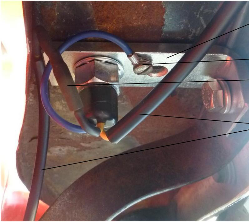
Brackets cut and drilled to fit from 1/4" x 1-1/4"- section heavy duty shelf brackets from hardware store.
