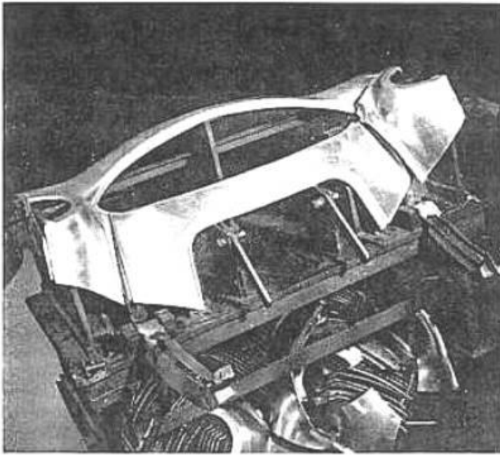
The four small sections which make up the nose sub-assembly, before the welding jig is closed
