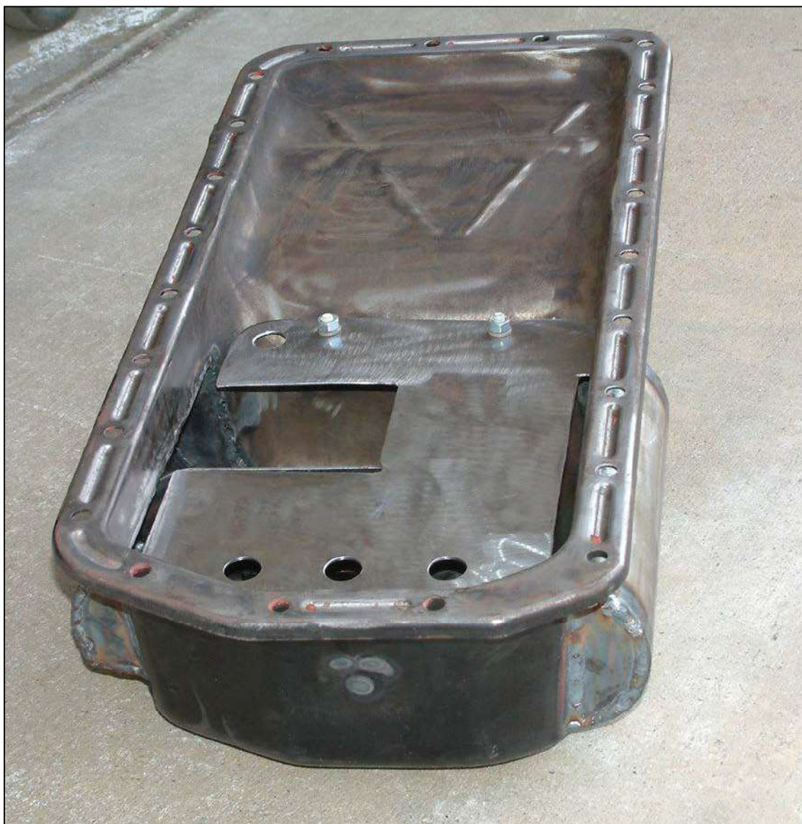
Above: The completed GT-6 oil pan with splash plate and extensions on the side to increase the capacity of the pan as described in the text.
