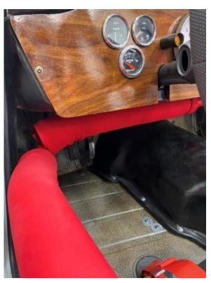
The race interior features an oil pressure, water temperature and voltage gauges with a Summit Racing tachometer. Controls include a pushbutton starter and fused toggle switches. The custom-covered (removable and washable) padded 6-point roll bar is a bolt-in unit and a 4-panel rearview mirror is mounted on the dash. A Corbeau racing seat with a harness is included. The car has undergone a fresh repaint in white with red accent highlights on the front valance and both side rockers.
