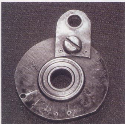
Below: Larger-diameter cam made by Kas with sealed ball bearing in centre. The tab for connecting to the throttle linkage is quickly detachable for easy adjustment
