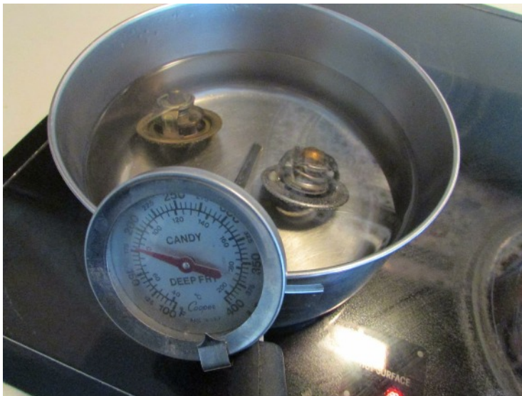
Stat on right starting to open at 180°.
