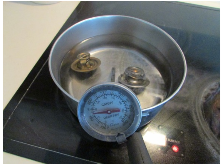
Old stat on left partially open at 170°.
